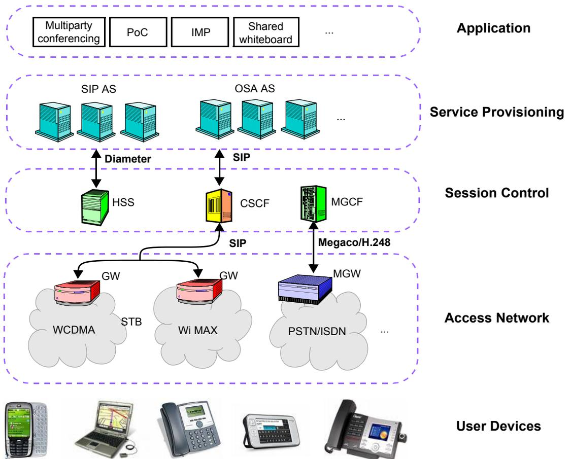
Figure 1. IMS layered architecture from the application servers to the user devices.
