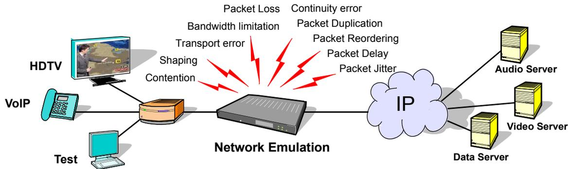
**Figure 6.** ALBEDO Net.Storm is the selected network impairments generator that allows to simulate the network
