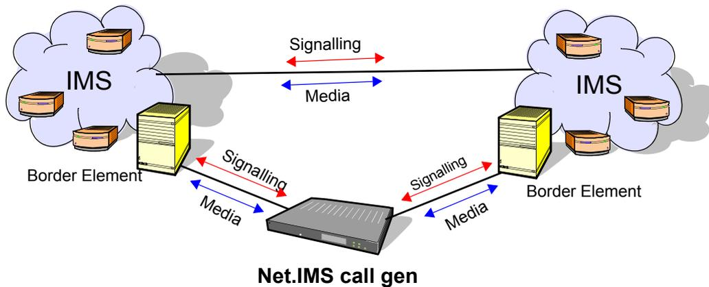
**Figure 4.** Net.IMS call gen can generate numerous call/session profiles across numerous protocols simultaneously, allowing it to simulate a wide variety of real and unusual traffic patterns.
