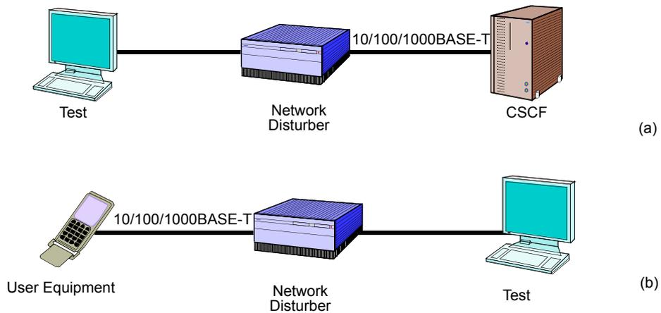
Figure 3. Extra test scenarios for media quantity verification: (a) Setup E, checks the network end of the Gm interface with custom network impairments. (b) Setup F, is similar to setup E but it is adapted to check the user-Gm interface.
