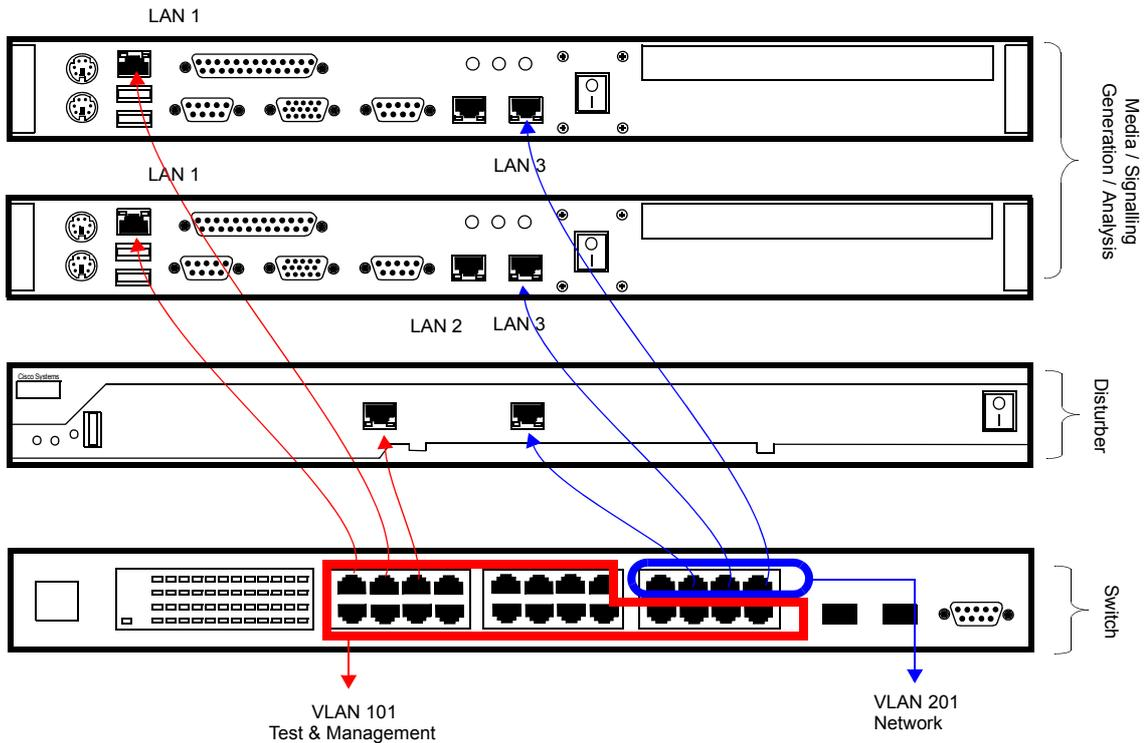
Figure 5. Preliminary block diagram for the IMS laboratory.
