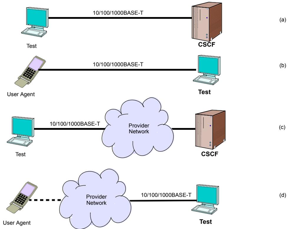
**Figure 2.** Tests scenarios for verification of the Gm interface (a) Setup A, checks the Gm-Network interface, (b) Setup B, checks the Gm-User interface, (c) Setup C, similar to scenario A but it integrates the provider access network within the system under test, (d) Setup D, similar to scenario B but it integrates the provider access network within the system under test.
