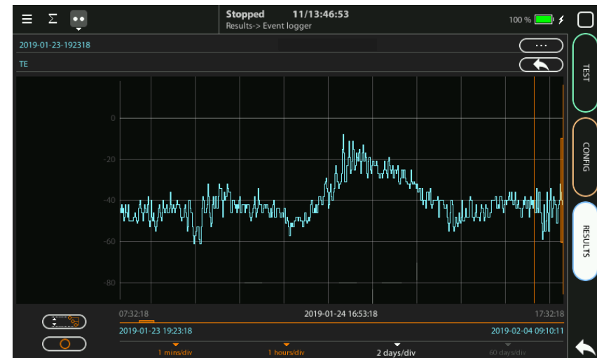
Phase Time Error extracted from captured SV
