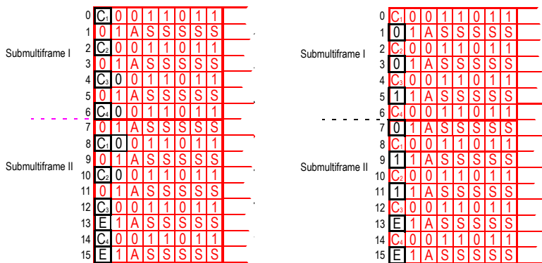
Figure 1.13 The CRC-4 provides error monitoring by means of four Ci bits that correspond to the previous submultiframe. If the receiver detects errors, it sets the E-bit to indicate the error. The “001011” sequence is used to synchronize the submultiframe.
