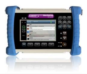
Ether-DuaLoop is a battery operated loop-back device with two optical/electricalports that can be work independently looping back Ethernet/IPL1-L4 packets used to execute acceptance and assurance tests including RFC2544 or eSAM.
