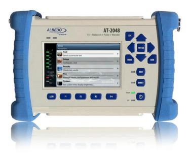
The AT-2048 is a tester specifically designed in 2011 for field engineers installing, commissioning and trouble-shooting E1, Datacom, Wander, Frame Relay services.
