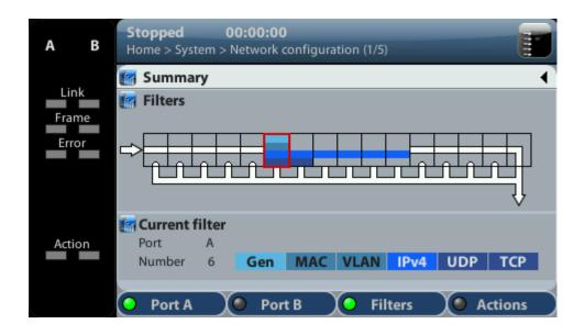
Net. Hunter is equipped with 16 filters to capture traffic in real time
