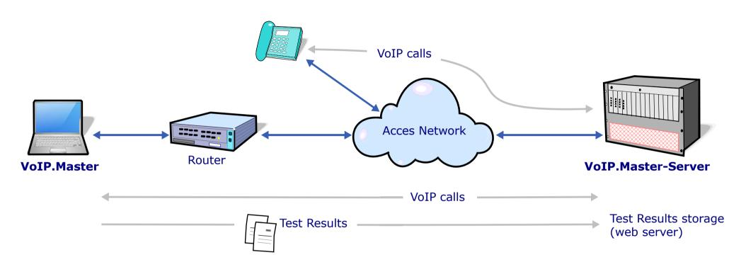
This is **centralized version** which is based on a Server that can work with VoIP. Master or directly with VoIP terminals to improve test process and increase technician efficiency and productivity:
