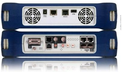
**Zeus** provides deep insights to design, install, maintain, troubleshoot and engineer communications infrastructures of the Smart Grid and more particularly of the Power Substations. The unit is able to test Ethernet/IP, PTP, GbE, IRIG-B, T1/E1, G703, C37.94, GOOSE, SV and MMS protocols. One-way-delay tests, assisted by GPS, is possible at all interfaces.
