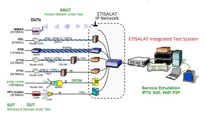
Figure 5. It is also possible to Implement ETISALT network in order to verify the quality of the services and access network
