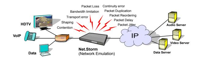
Figure 10. ALBEDO Net.Storm is the selected network impairments generator that allows to Implement the network
