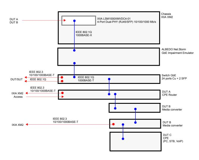
Figure 4. Block diagram of some elements of the Integrated Multimedia Test System (IMTS).
