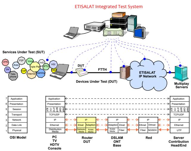
**Figure 2.** The model of seven levels of telecommunications allows the router, not have to analyse the payload of the IP frames, or what is the same, never engages with the upper levels of protocols or applications.
