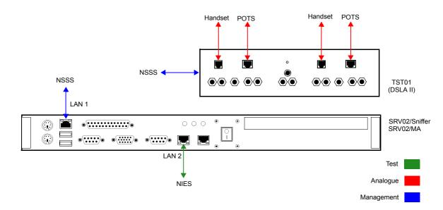
**Figure 6.** The TGAS is made up by two different devices, the TST01 generates different kinds of test analogue audio signals. The SRV02/MA is a software installed in the SRV02 that generates and analyses test VoIP signals.
