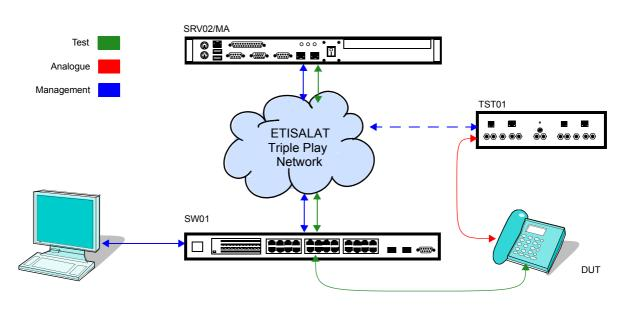
Figure 7. Typical test setup that makes use of the TGAS.
