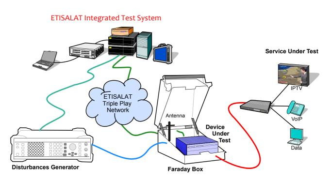
Figura 14. An interfering signal in the frequency band in which you want to create disturbance in the physical environment. The equipment being measured (DUT) is inserted into the suitcase of Faraday. If it were a router, as the case illustrated in Figure, first access network to the test system and on the other client computers using the appropriate physical environment Coax, UTP or PLC. In the case of WiFi transmitter and receiver must be placed inside the Faraday Box.
