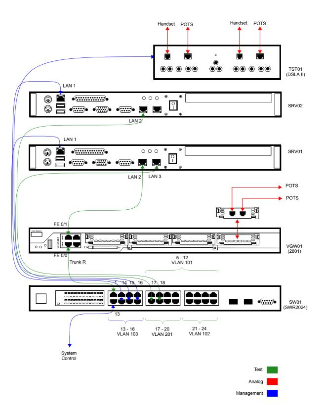
Figure 15. ALBEDO Integrated VoIP Lab to execute conformity and acceptance test procedures for VoIP terminals, PBX and systems.
