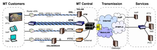
**Figure 4.** Actual and possible evolution of the Network of MT regarding advanced services over IP combining DSLAM and MSAN in the same network to provide Multiplay services including VoIP, IPTV, Data, and High Speed Internet.
