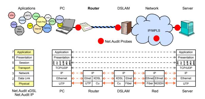
Figure 7. Net. Audit is focused on remote monitoring of the QoS at IP layer-3 while Net. Audit xDSL is focused on remote test a prequalification of the copper layer 1 used for ADSL, ADSL2 and ADSL2+ and VDSL2 access.
