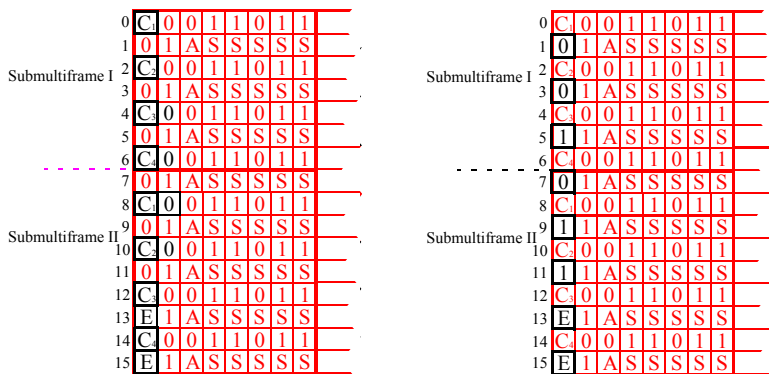
Figure 14 The CRC-4 provides error monitoring by means of four C_i bits that correspond to the previous submultiframe. If the receiver detects errors, it sets the E-bit to indicate the error. The “001011” sequence is used to synchronize the submultiframe.
