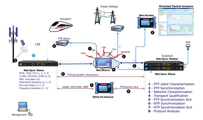
Figure 1 PTP benchmarking solution to conduct approval and acceptance test suites.
