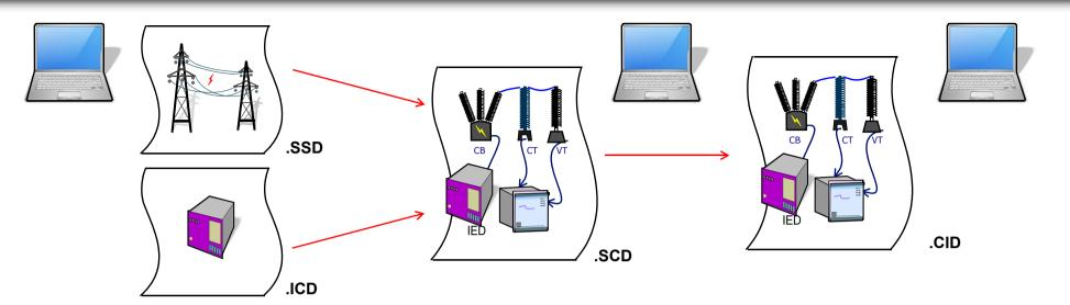
The **Substation Configuration Language** (SCL) specified by IEC 61850 for the configuration of substation includes representation of modeled data to have a complete interoperability:
