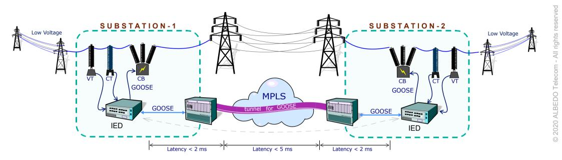
GOOSE is a Layer 2 protocol (not routable) used by IEDs send messages inside the substation LANs, nevertheless using MLPS it can be extended to remote substations and Tele-protection. MPLS facilitates GOOSE traffic through the WAN extending the LAN thus IEDs can exchange information with remote devices at remote substations:
