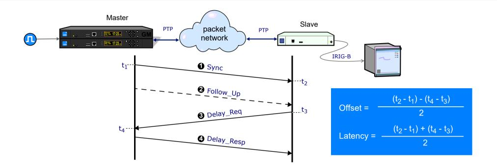
It is a cost-efficient solution and can be applied on the basis of the existing Ethernet network in a substation. PTP (IEEE 1588) applies master/slave time synchronization mechanisms and supports hardware time stamps. The basic parameters of Latency / Offset are computed from the t<sub>1-4</sub> stamps.
