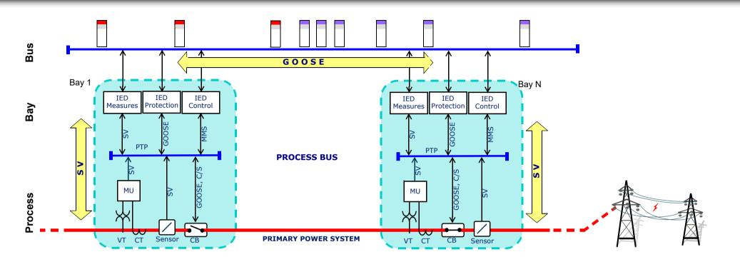
During normal operating conditions IED broadcast and retransmits GOOSE messages cyclically, this is the **heartbeat** of the substation. The health of the GOOSE messages are monitored closely to assure on-time delivery. A missing message is an indication for the **Subscribers** that the communication from the **Publisher** has become disturbed.
