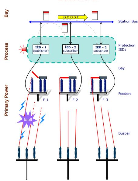
A fault causes a voltage drop on a feeder and, after the clearing of the fault, results in an inrush condition (a sudden arrival of energy) which may lead to a undesired operation of protection on the healthy feeders.
