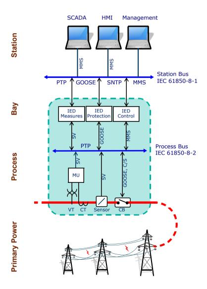
GOOSE is a messaging system used by IEDs and mission-critical applications to tell about substation substation events, such as commands, alarms, indications and measurements:
