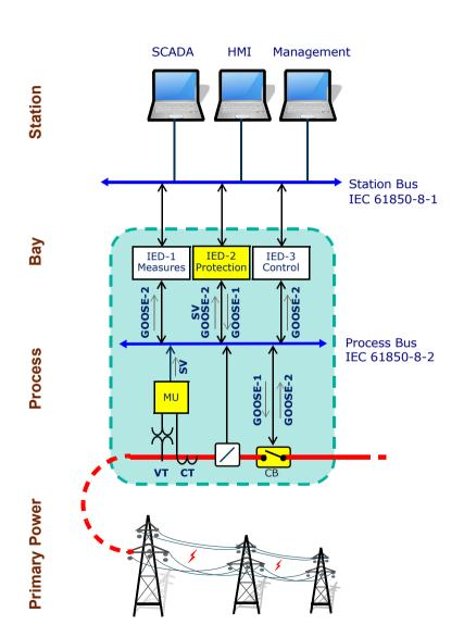
A **Merging Unit** (MU) accepts multiple analogue current and voltage samples coming from the VT and CT current and voltage transformers which are connected directly to the power line.
