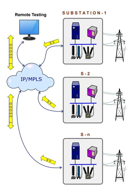
Since IEC 61850 Edition 2 – the **Simulation bit** in the GOOSE message and the different modes of the tested function elements play a critical role in the verification of Utility systems including the ability to **remotely test** a subset of functions and their elements while keeping the rest of **the system in service**.
