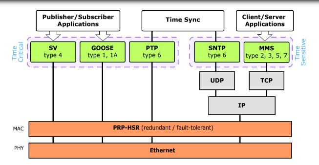
The IEC 61850 is a set of standards and technical reports for interoperability (between devices and systems), ease of configuration (allocation of functions to devices), long term stability (layered, object-model based design), and reliability (lossless network architectures) to replace wire communications.
