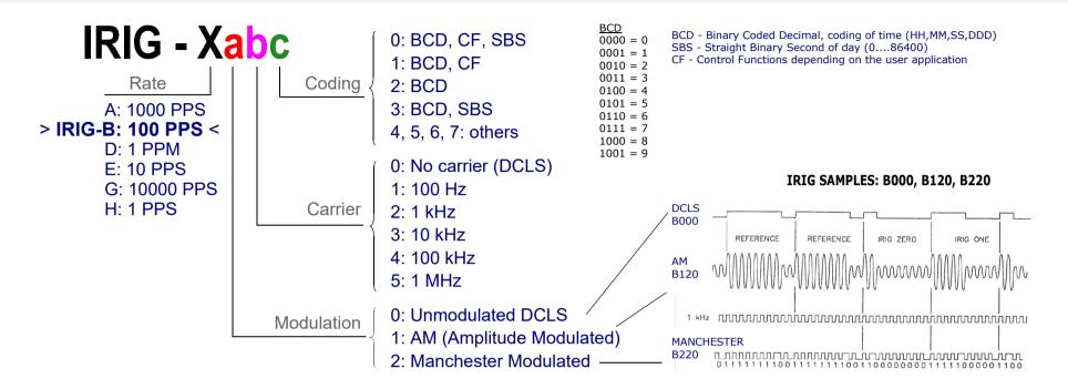
IRIG-B sends a timing signal every second at 100 pulse/sec rate therefore the 100 is the number of bits of each frame. IRIG-B info includes Year, Day of the year, Hour, Min and Sec.
