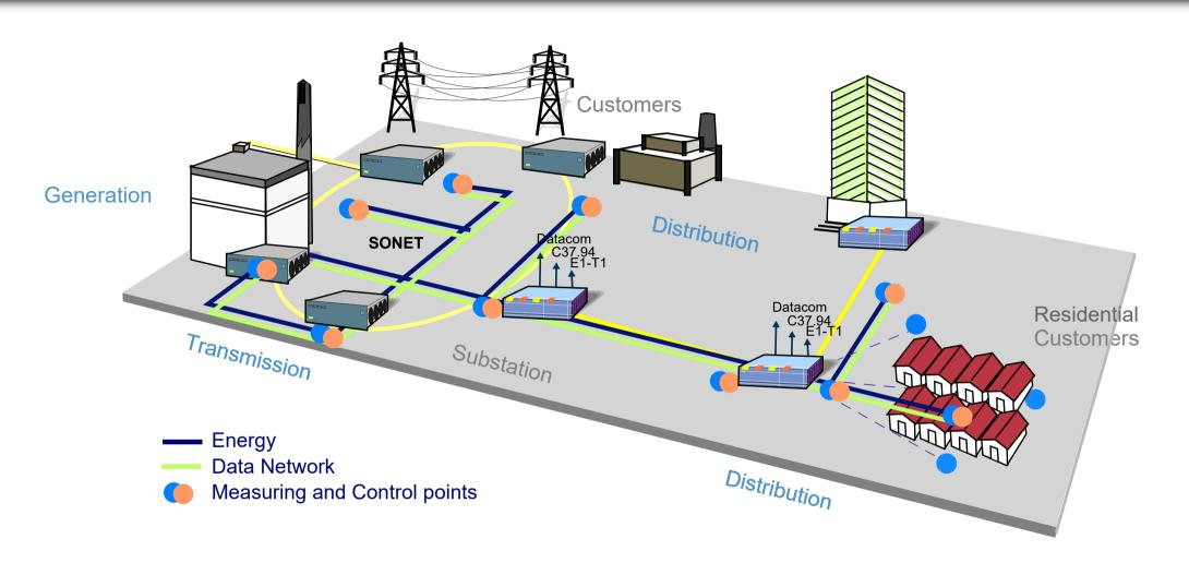
Smart Grid require a **Telecom Data Network** to communicate all the elements of the Power System, including Generation plants, Substations and Customers in order to increase the efficiency, resilience and quality of the power grid, while allowing advanced management.
