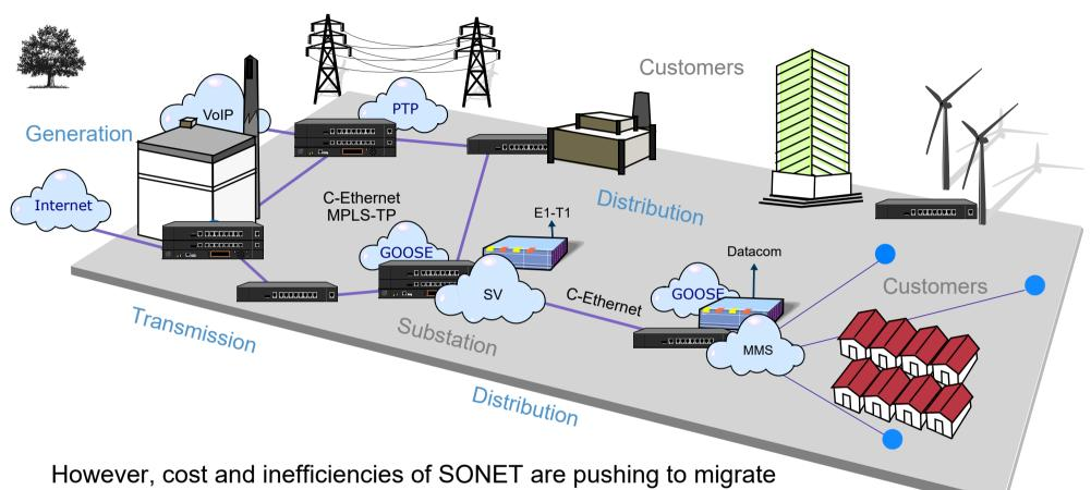
However, cost and inefficiencies of SONET are pushing to migrate towards Carrier-Ethernet or MPLS in the WAN whilst in the substation to the IEC 61850 in order to integrate all data traffic generated at the power grid under the Ethernet umbrella:
