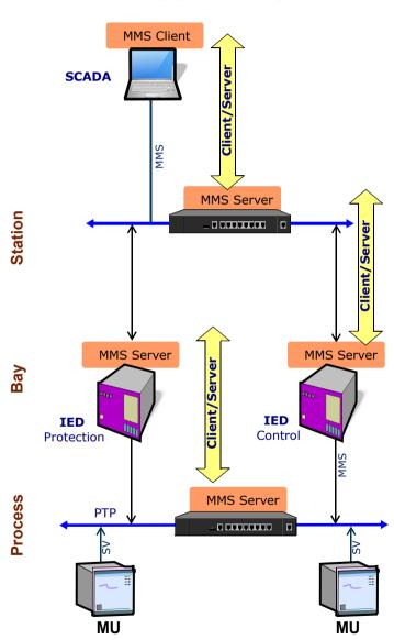
MMS is used by the applications to **transfer data** between substation levels, communicating IEDs and SCADA systems to move the information such as device status, obtain reports, data acquisition in order to monitor and get control.
