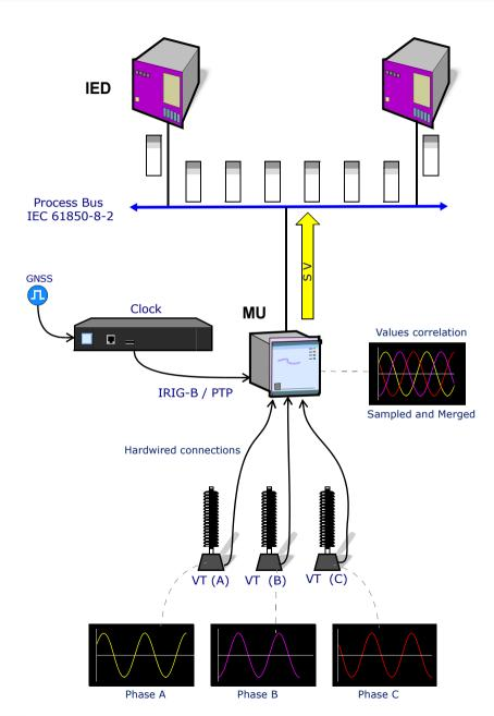
A **Merging Unit** (MU) is an IED that digitizes the analog measurements taken by current and voltage transformers. Afterwards the MU publishes the data as a stream at a predefined rate.
