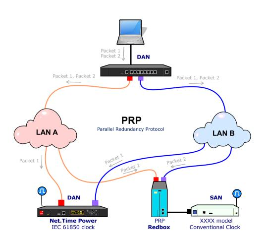
PRP is based on the use of two independent networks. The sender **must send each packet twice** (to LAN A and LAN B) through two separate ports.
