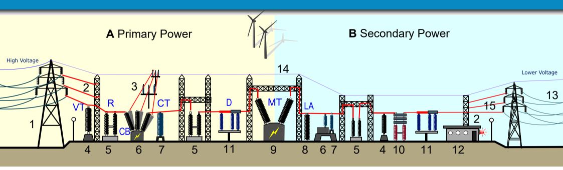
1.Primary Power (PP), 2.Feeder, 3. Busbar, 4.Voltage Transformer (VT), 5.Relay (R), 6.Circuit Breaker (CB), 7.Current Transformer (CT), 8.Lightning Arrester (LA), 9.Main Transformer (MT), 10. Capacitors (C), 11.Disconnector, 12.Control Shelter, 13.Secondary Lines, 14. Ground, 15. Overhead Lines
