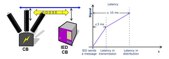
The performance of hardwired solutions is based on relays that in the worst scenario the IED transfer time can be 3/4 of cycle (15ms) that is improved with GOOSE alternative below to 3 ms.
