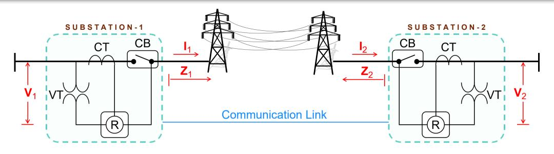
There are several line Protection schemes based on the measurement of electric values:
