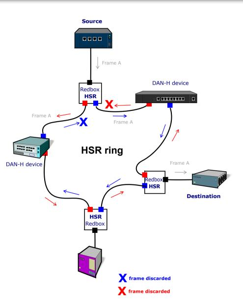
High-availability Seamless Redundancy (**HSR**) provide **seamless failover** from a single point of failure. HSR is designed primarily for ring topologies.
