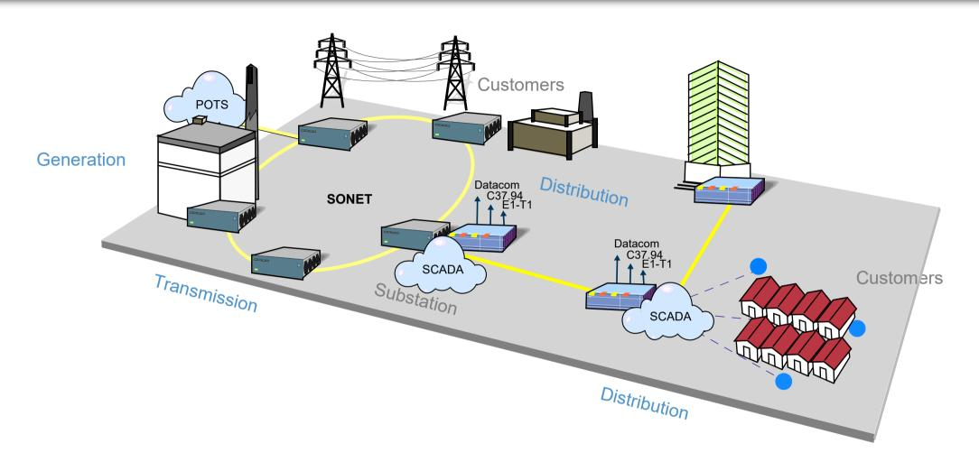
At the 80's SONET was the first network to be deployed and it was a satisfactory solution for common applications such as SCADA, Telephony and Tele-protection because it is a predictable, symmetric, low latency, and fault tolerance architecture.
