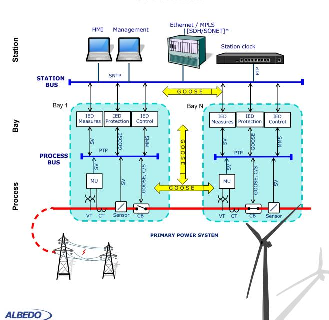
GOOSE most often applications is used for **protection**, **control and automation** of electric systems.
