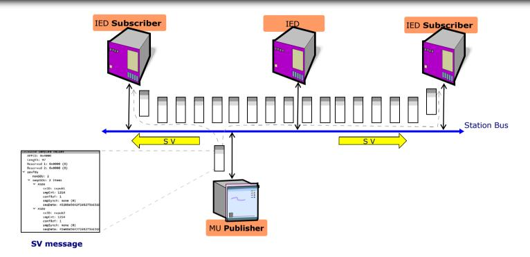
It is defined in the standard to provide a fast and cyclic transfer of samples.
