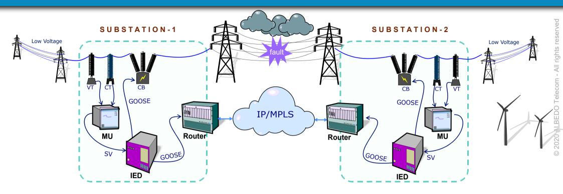
Each protection IED analyses the SV data from MU and transmits GOOSE messages containing the trip status. The "smart" circuit breakers are responsible for subscribing to the appropriate relay trip GOOSE messages to actuate after the trip data attribute is set.
