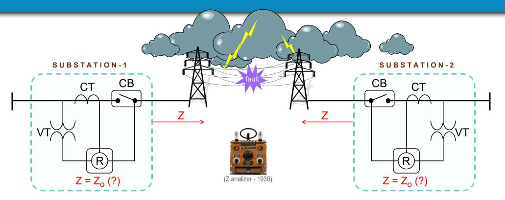
Impedance **Z = V / I** that is obtained measuring Voltage (V) at VT and Current (I) at CT.
