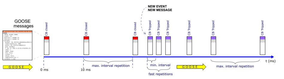
Since the GOOSE messages replace hard-wired signals used for protection and control applications IEC 61850 introduces mechanisms that ensure the delivery of the required information.
