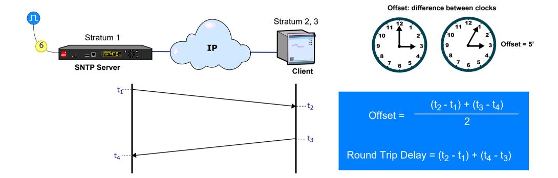
SNTP is part of the IEC 61850 standard (a simplified version of NTP) which can provide a milisecs range of precision, is good enough for the station bus to synchronize SCADA and Ethernet switches but is not for the Process Bus with GOOSE and SV messages and devices that require an accuracy of microsecs.
