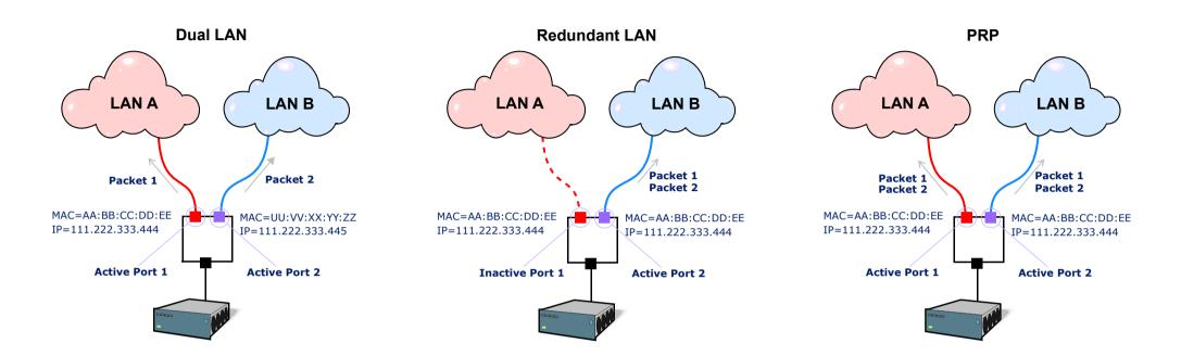
PRP is based on the use of two independent networks: LAN A & LAN B
