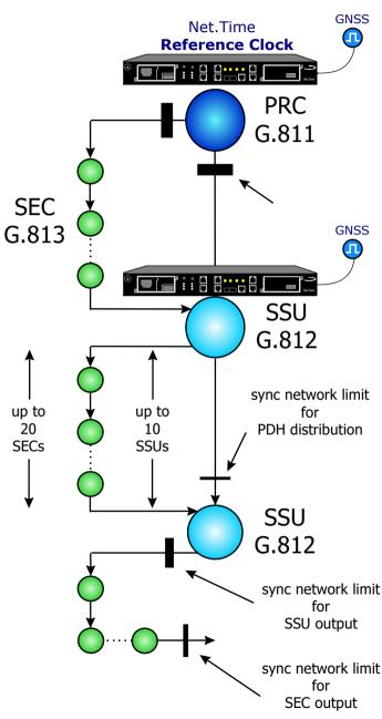
Net.Time configured as PRC is equipped with Rubidium oscillator providing timing to the SSU that can be a Net.Time with OCXO oscillator.
