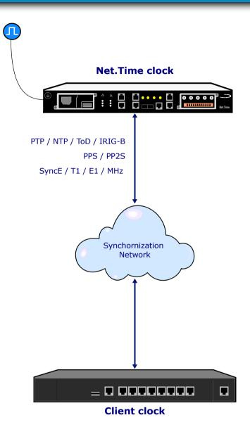
Net. Time can synchronize by means of several signals that can be grouped according the following hierarchy.
