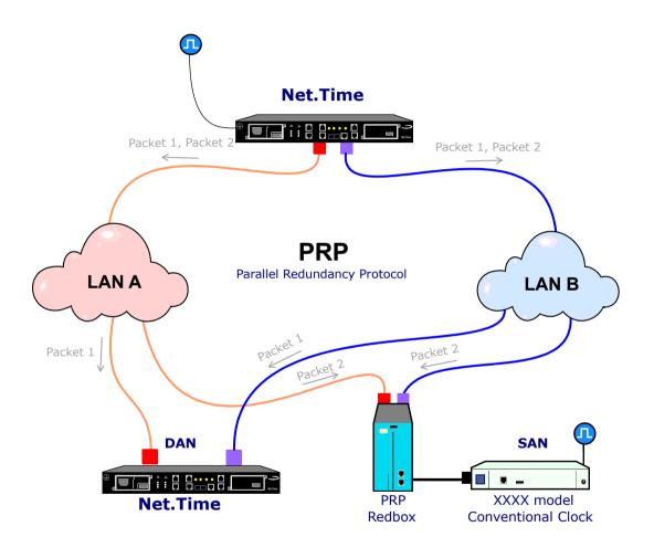
PRP is based on the use of two independent networks. The sender must send each packet twice (to LAN A and LAN B) through two separate ports. There are two types of devices:
