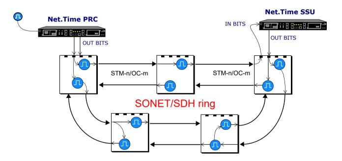
Often known as Building Integrated Timing Supply (BITS) there are several signals suitable for transporting synchronization:
