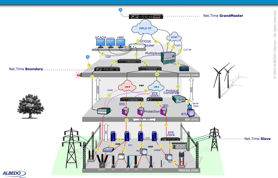
Many Utilities acquire timing from GNSS and the station clock converts signal into a 1-pps or IRIG-B code, which are then distributed by dedicated links to all the IEDs in a substation. However, important to say that this system has some **weaknesses** (\*) being **vulnerable** to human and natural disruptions that may perturb normal operations by raising false alarms, delaying actions, and lowering system efficiency.
