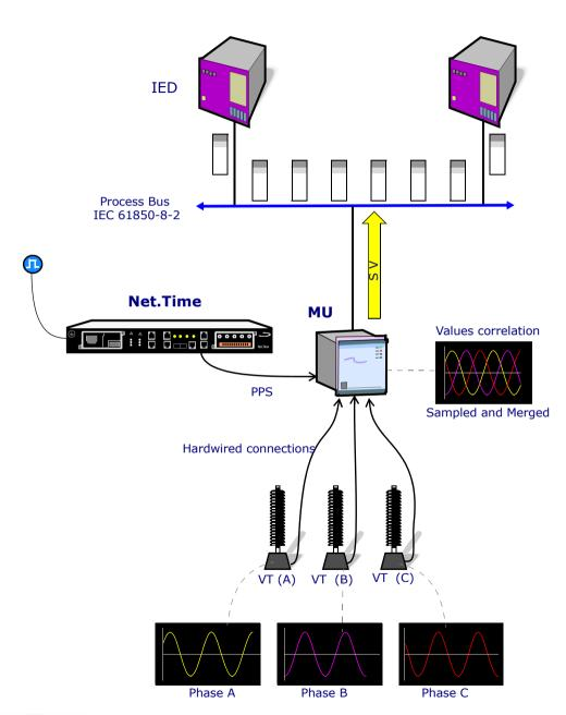
Merging Units (MU) require **Phase Synchronization**. MU digitize analog measurements of current / voltage.
