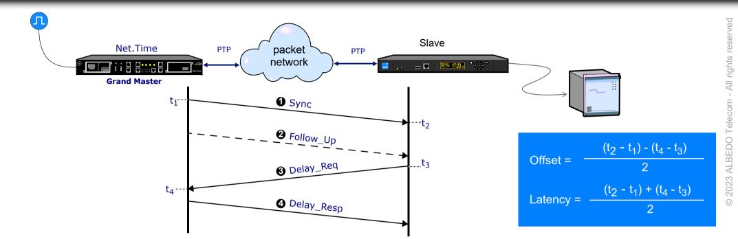
It is a cost-efficient solution and can be applied on the basis of the existing Ethernet network in a substation. PTP (IEEE 1588) applies master/slave time synchronization mechanisms and supports hardware time stamps. The basic parameters of Latency / Offset are computed from the  $t_{1...4}$  stamps.
