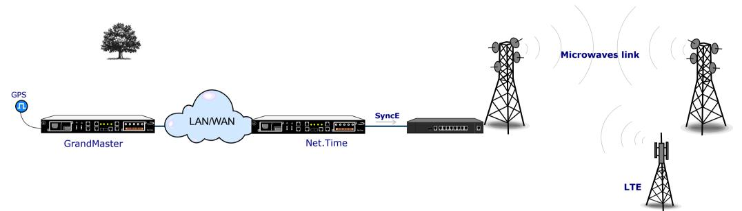
Net. Time supports Synchronous Ethernet over a copper and optical connections. This allows operators to utilize cables on SFP ports and still meet timing and synchronization requirements for demanding applications like LTE in mobile networks and microwaves links.
