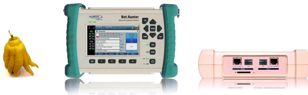
Figure 1 Net.Hunter is a stream-to-disk appliance capable of monitoring live traffic to capture and record selected TCP/IP flows at wirespeed. It includes an embedded tap with triggers and programmable filter conditions.
