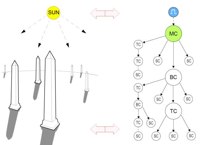
**Figure 4** A typical synchronization network has a tree architecture. At the root, a Master Clock (MC) sends PTP packets to the Slave clocks (SC) to discipline their oscillators. In the branches Boundary (BC) and Transparent Clocks (TC) regenerate and forward the signals. The result is a hierarchical topology with one MC and a number of BC, TC and SC.
