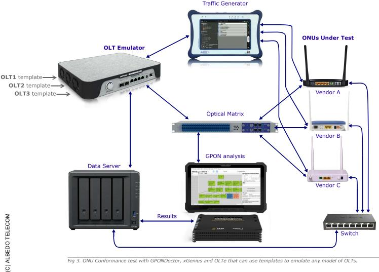
Fig 3. ONU Conformance test with GPONDoctor, xGenius and OLTe that can use templates to emulate any model of OLTs.
