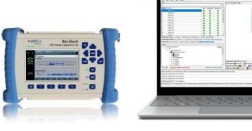
Solution for monitoring and commissioning a GOOSE installation, consisting of a Tap and a Protocol Analyser. The Tap filters and forwards messages to GOOSE Monitor, the application that displays the IED topology and the messages in real time.
