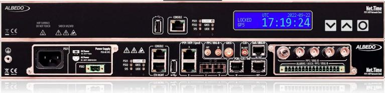
Net.Time GM manages the PTP in the WAN or in the Substation while Net.Edge multiplies the number of ports (x8) and may also adapt bit-rates (to 2,5 GbE) using a a 11 Gbps switch matrix.
