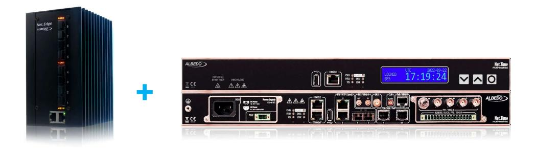
Net.Time is timing source while Net.Edge not only multiply the number of ports working a Transparent Clock (TC) or Boundary Clock (BC) but also forwards the PTP signal while correcting the path, ensuring on this way that downstream equipment always receives accurate and stable time.
