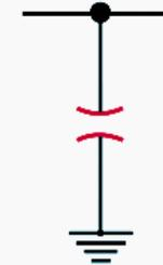
Lightning arrester (valve type)
