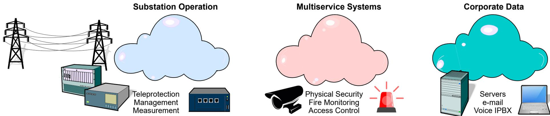
Communication infrastructures of a substation have three separate and differentiated networks:
