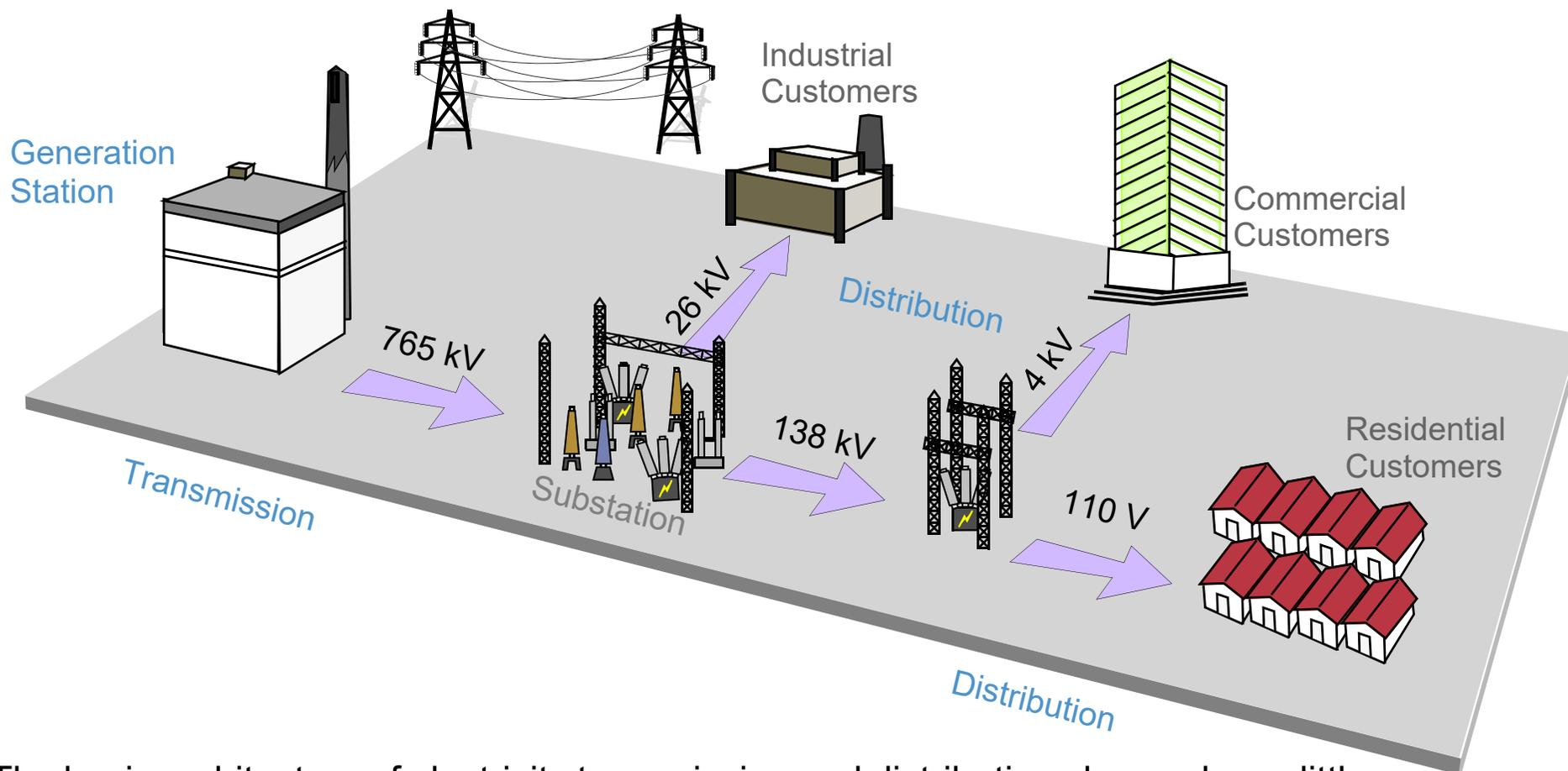
The basic architecture of electricity transmission and distribution changed very little during the first 100 years. However, in recent decades, the concept of **Smart Grid** emerged thanks to the massive use of digital technologies to increase efficiency, resilience and quality of the service.
