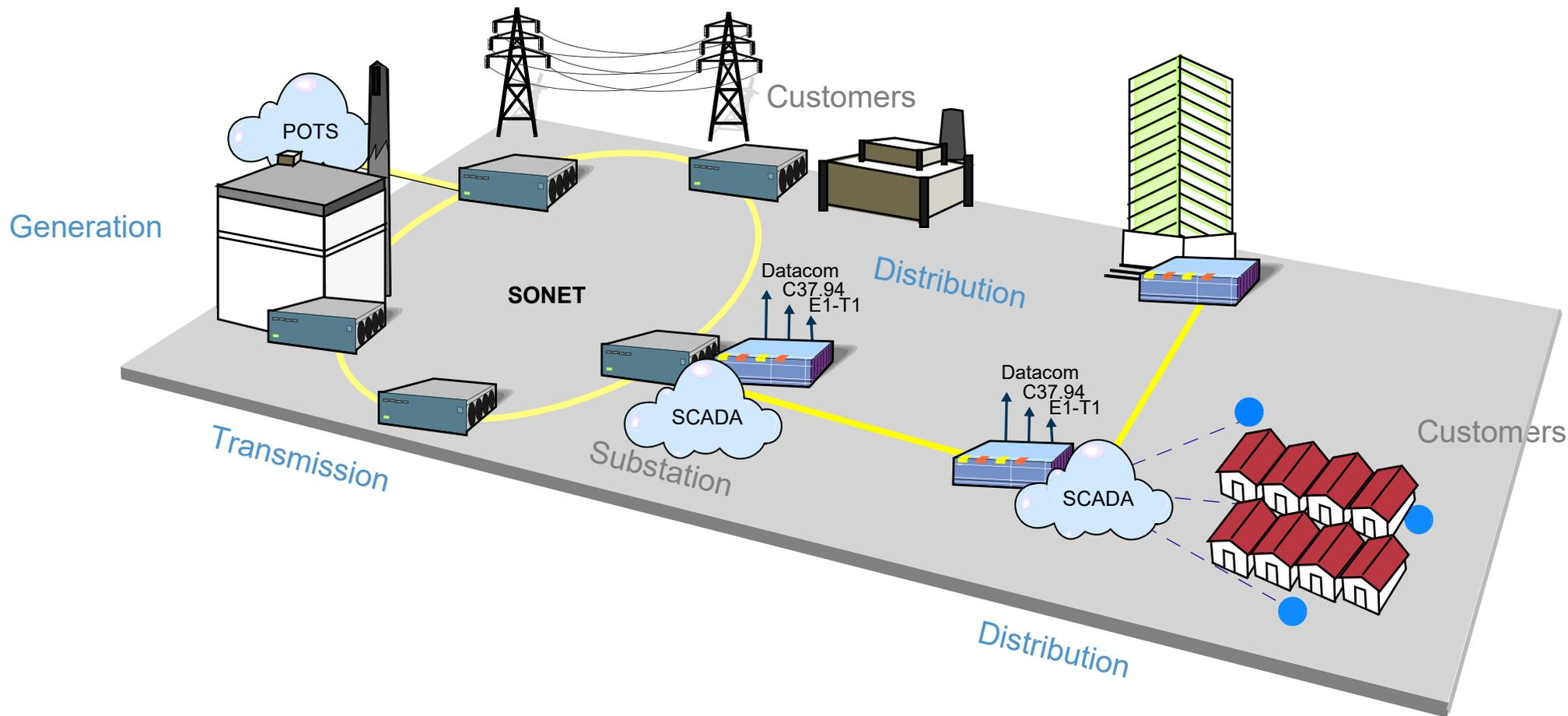
At the 80's SONET was the first network to be deployed and it was a satisfactory solution for common applications such as SCADA, Telephony and Tele-protection because it is a predictable, symmetric, low latency, and fault tolerance architecture.
