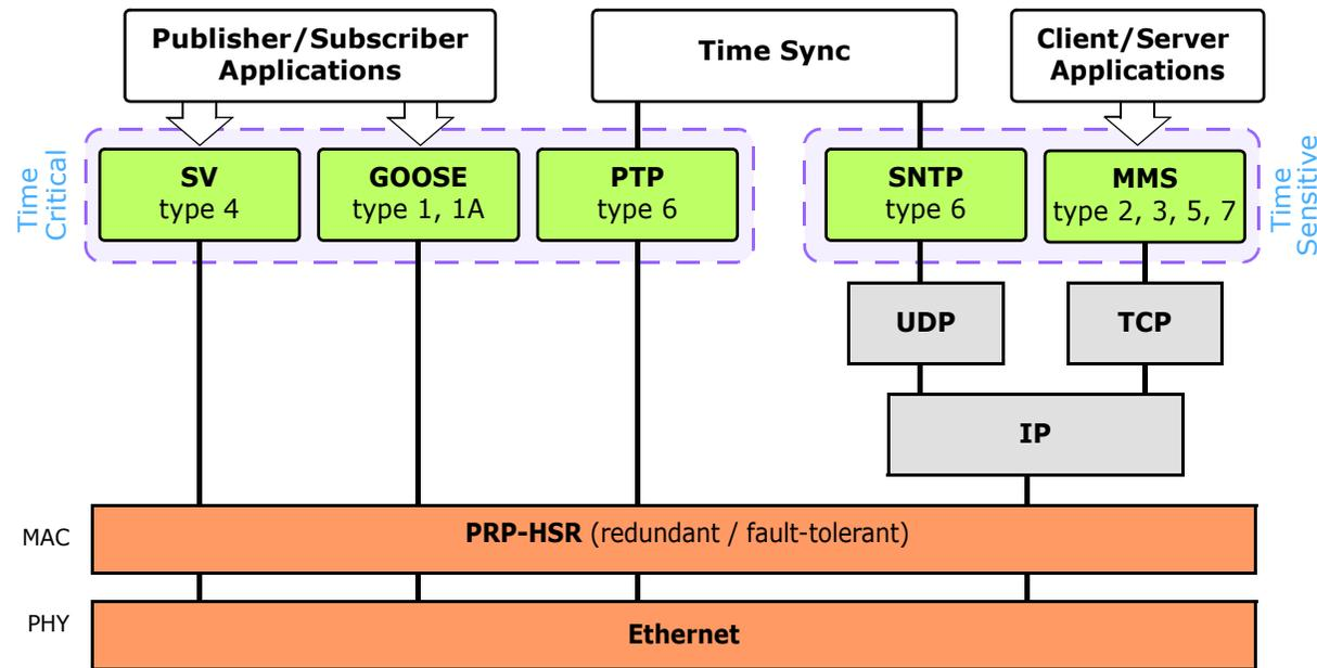
The IEC 61850 is a set of standards and technical reports for interoperability (between devices and systems), ease of configuration (allocation of functions to devices), long term stability (layered, object-model based design), and reliability (lossless network architectures) to replace wire communications.
