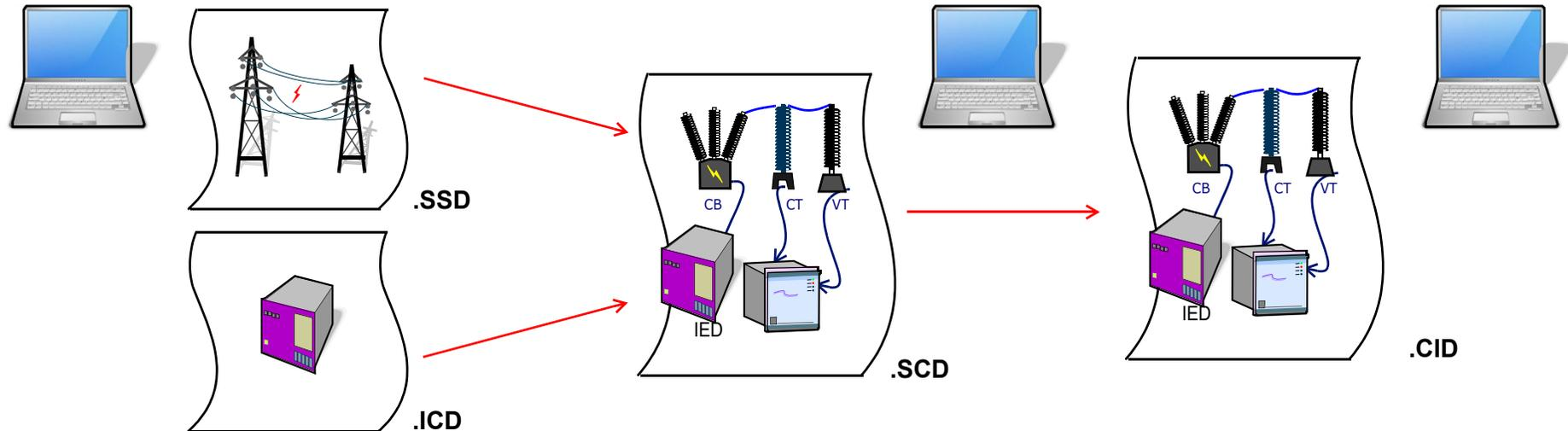
The **Substation Configuration Language** (SCL) specified by IEC 61850 for the configuration of substation includes representation of modeled data to have a complete interoperability:
