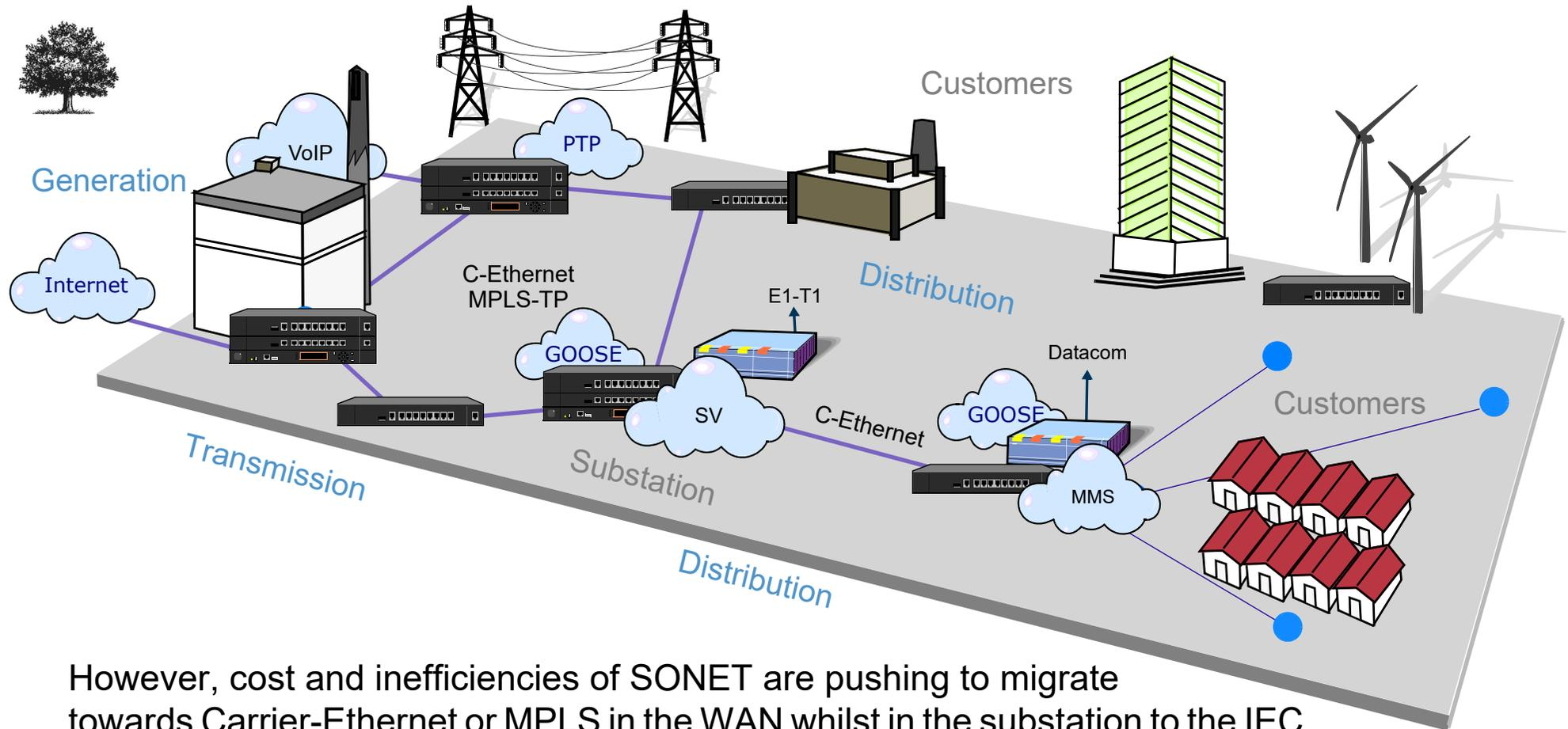
However, cost and inefficiencies of SONET are pushing to migrate towards Carrier-Ethernet or MPLS in the WAN whilst in the substation to the IEC 61850 in order to integrate all data traffic generated at the power grid under the Ethernet umbrella:
