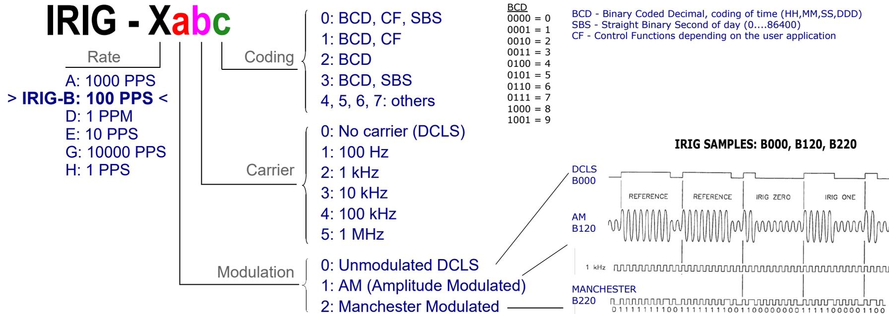
IRIG-B sends a timing signal every second at 100 pulse/sec rate therefore the 100 is the number of bits of each frame. IRIG-B info includes Year, Day of the year, Hour, Min and Sec.
