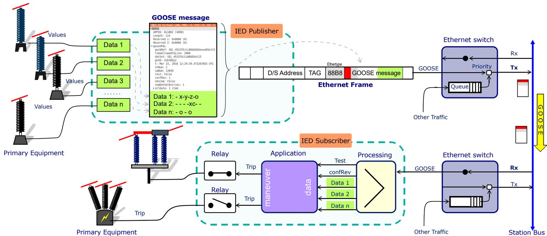
1. The IED publisher writes the values in a transmission buffer and multicast it over the substation local area network to the different subscribers sends the message without requirements and confirmation.
