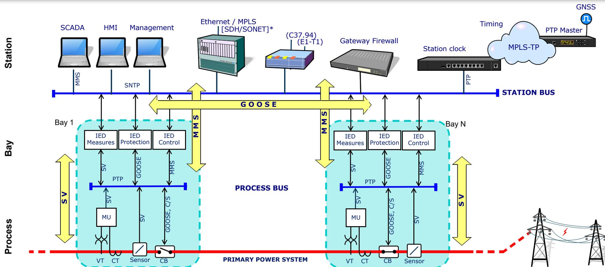
The **Station bus** provides connectivity to individual bays, distributed controllers, gateways, management and human machine interfaces (HMIs). It may connect up to hundreds of Intelligent End Device (IEDs), often segmented physically or logically depending on their application.
