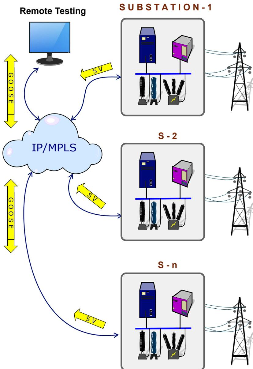
Since IEC 61850 Edition 2 – the **Simulation bit** in the GOOSE message and the different modes of the tested function elements play a critical role in the verification of Utility systems including the ability to **remotely test** a subset of functions and their elements while keeping the rest of **the system in service**.
