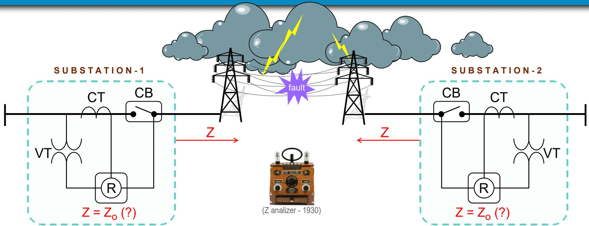
Impedance  $Z = V / I$  that is obtained measuring Voltage (V) at VT and Current (I) at CT.
