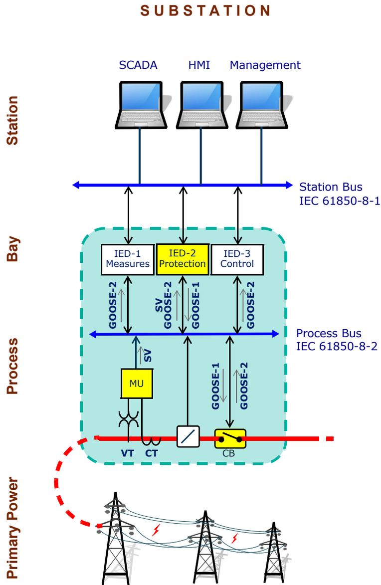
A **Merging Unit (MU)** accepts multiple analogue current and voltage samples coming from the VT and CT current and voltage transformers which are connected directly to the power line.
