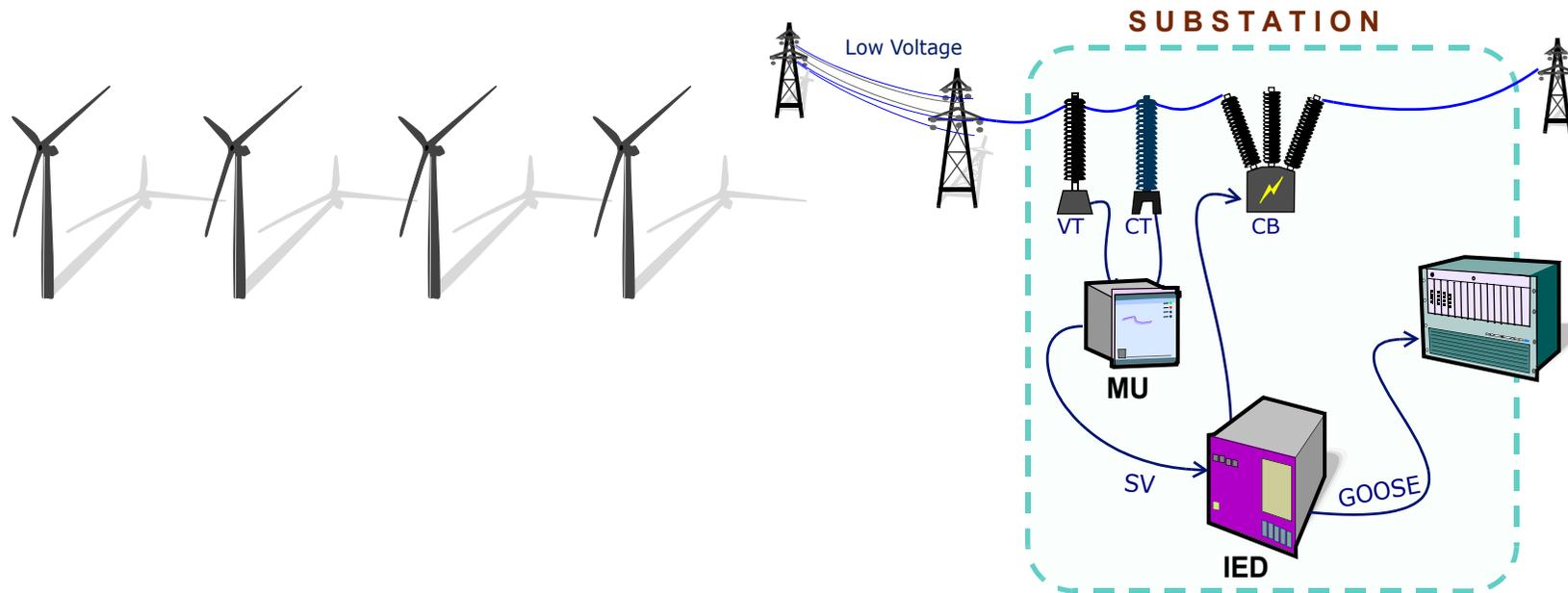
**Sampled Values (SV)** or **Sampled Measured Values (SMV)** is a protocol defined in IEC 61850-9-2 for the acquisition of raw data [8]. In particular, it facilitates the transfer of digitized samples of analog measurements. SV is time critical and can be streamed as unicast or multicast.
