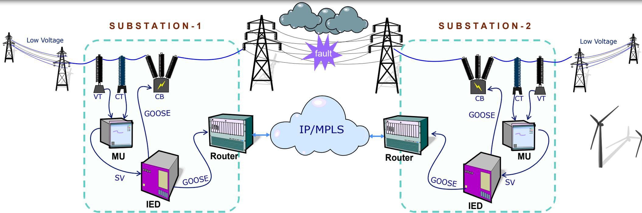
Each protection IED analyses the SV data from MU and transmits GOOSE messages containing the trip status. The “smart” circuit breakers are responsible for subscribing to the appropriate relay trip GOOSE messages to actuate after the trip data attribute is set.
