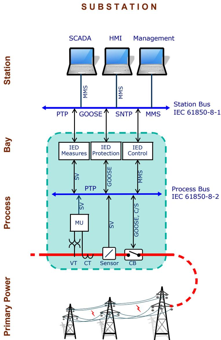
GOOSE is a messaging system used by IEDs and mission-critical applications to tell about substation substation events, such as commands, alarms, indications and measurements:
