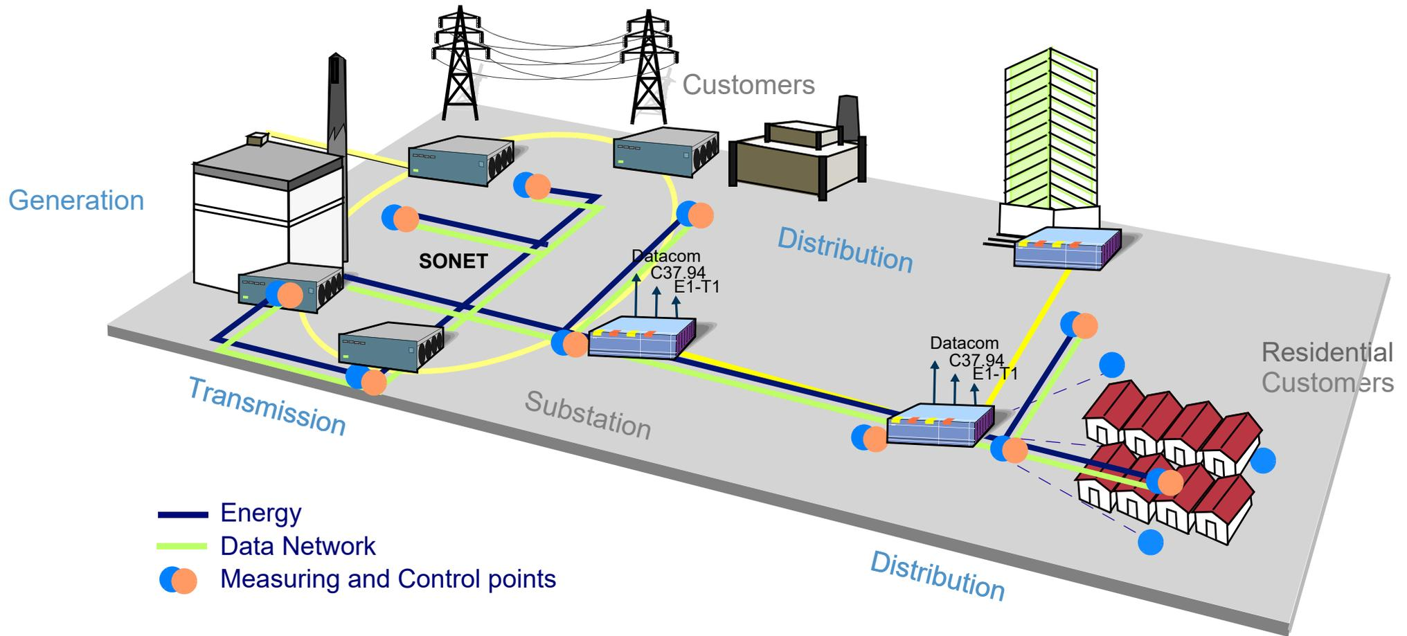
Smart Grid require a **Telecom Data Network** to communicate all the elements of the Power System, including Generation plants, Substations and Customers in order to increase the efficiency, resilience and quality of the power grid, while allowing advanced management.
