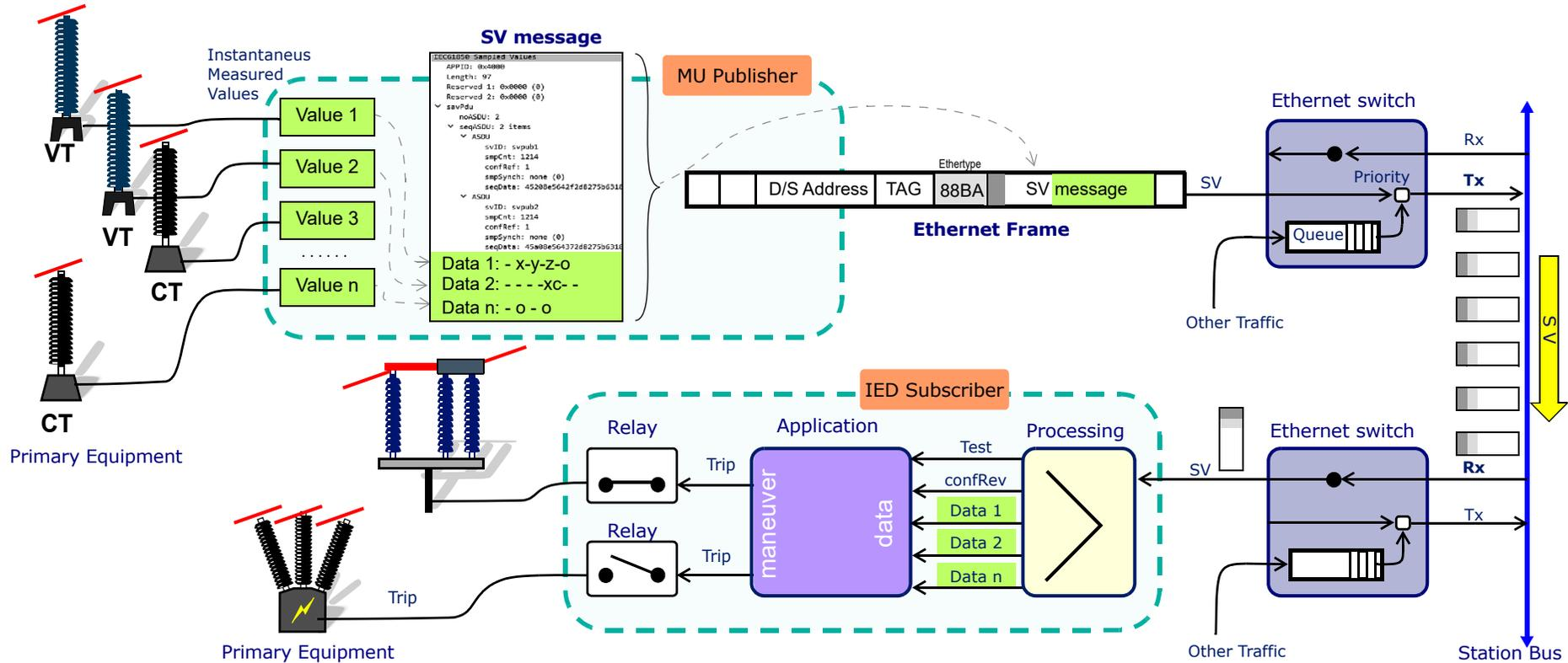
1. Merging Units digitalize the values and build the SV message mapped in Ethernet frames
