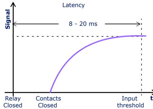
The performance of hardwired solutions is based on relays that in the worst scenario the IED transfer time can be 3/4 of cycle (15ms) that is improved with GOOSE alternative below to 3 ms.
