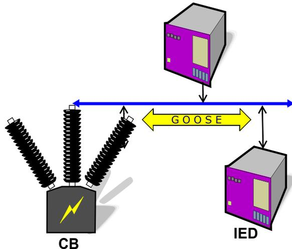
1. **Installation Costs:** due to the replacement of thousands individual control copper cables with a limited number of fiber optic cables from the terminal blocks to the relay terminals with a single pair of fiber.
